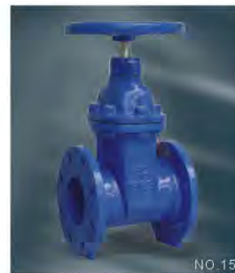
Non rising stem resilient soft seated gate valves BS 5163
